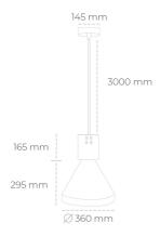
COB Light colour 2700 [K] | CRI Led chip flux 3772 [lm] 3394 [lm] Luminous flux System power 27 [W] Luminaire Efficiency 126 [lm/W] Beam angle 45° Controller ON/OFF MacAdam 3 SDCM
