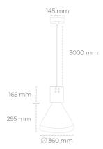
COB 3000 [K] CRI97 Light colour CRI 3368 [lm] Led chip flux Luminous flux 3031 [lm] System power 31 [W] Luminaire Efficiency 98 [lm/W] Beam angle 15° Controller ON/OFF
