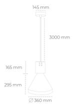
COB 4200 [K] MEAT WHITE Light colour CRI 90 Led chip flux 2695 [lm] Luminous flux 2425 [lm] System power 27 [W] Luminaire Efficiency 90 [lm/W] Beam angle 60° Controller ON/OFF MacAdam 3 SDCM
