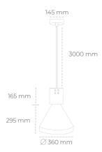
COB Light colour 3500 [K] | CRI Led chip flux 2783 [lm] Luminous flux 2504 [lm] System power 19 [W] Luminaire Efficiency 132 [lm/W] Beam angle 15° Controller ON/OFF MacAdam 3 SDCM
