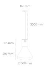
COB 4200 [K] MEAT WHITE Light colour CRI 90 Led chip flux 2519 [lm] Luminous flux 2267 [lm] System power 25 [W] Luminaire Efficiency 91 [lm/W] Beam angle 38° Controller ON/OFF MacAdam 3 SDCM
