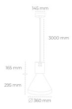
COB 3500 [K] HI EFFICIENT Light colour CRI 90 Led chip flux 4181 [lm] Luminous flux 3762 [lm] System power 27 [W] Luminaire Efficiency 139 [lm/W] Beam angle 23° Controller ON/OFF MacAdam 3 SDCM
