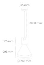
2500 [K] BREAD Light colour CRI 2808 [lm] Led chip flux Luminous flux 2527 [lm] System power 23 [W] Luminaire Efficiency 110 [lm/W]
