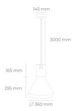
COB 3000 [K] HI EFFICIENT Light colour CRI 90 Led chip flux 4378 [lm] Luminous flux 3940 [lm] System power 27 [W] Luminaire Efficiency 146 [lm/W] Beam angle 45° Controller ON/OFF MacAdam 3 SDCM
