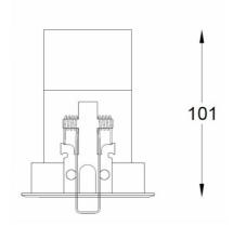
COB 2500 [K] BREAD Light colour CRI Led chip flux 1195 [lm] Luminous flux 956 [lm] System power 10 [W] Luminaire Efficiency 96 [lm/W] Beam angle 40° Controller ON/OFF MacAdam 3 SDCM
