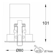
COB 4000 [K] HI EFFICIENT Light colour CRI 90 Led chip flux 1625 [lm] Luminous flux 1300 [lm] System power 10 [W] Luminaire Efficiency 130 [lm/W] Beam angle 40° Controller ON/OFF MacAdam 3 SDCM
