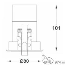
COB 3500 [K] HI EFFICIENT Light colour CRI 90 Led chip flux 2174 [lm] Luminous flux 1739 [lm] System power 14 [W] Luminaire Efficiency 124 [lm/W] Beam angle 40° Controller ON/OFF MacAdam 3 SDCM
