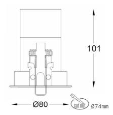
COB 2500 [K] BREAD Light colour CRI Led chip flux 1195 [lm] Luminous flux 956 [lm] System power 10 [W] Luminaire Efficiency 96 [lm/W] Beam angle 28° Controller ON/OFF MacAdam
