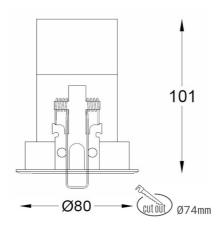
COB 3000 [K] CRI97 Light colour CRI Led chip flux 1144 [lm] Luminous flux 915 [lm] System power 10 [W] Luminaire Efficiency 92 [lm/W] Beam angle 28° Controller ON/OFF MacAdam 3 SDCM
