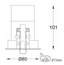
COB 3500 [K] HI EFFICIENT Light colour CRI 90 Led chip flux 2174 [lm] Luminous flux 1739 [lm] System power 14 [W] Luminaire Efficiency 124 [lm/W] Beam angle 28° Controller ON/OFF MacAdam 3 SDCM
