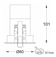
COB 3000 [K] HI EFFICIENT Light colour CRI 90 Led chip flux 2256 [lm] Luminous flux 1804 [lm] System power 14 [W] Luminaire Efficiency 129 [lm/W] Beam angle 28° Controller ON/OFF MacAdam 3 SDCM
