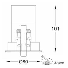
COB 3000 [K] CRI97 Light colour CRI Led chip flux 1144 [lm] Luminous flux 915 [lm] System power 10 [W] Luminaire Efficiency 92 [lm/W] Beam angle 18° Controller ON/OFF MacAdam 3 SDCM
