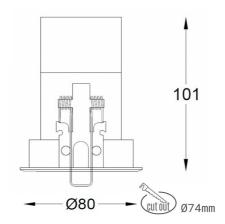
COB 4000 [K] HI EFFICIENT Light colour CRI 90 Led chip flux 1625 [lm] Luminous flux 1300 [lm] System power 10 [W] Luminaire Efficiency 130 [lm/W] Beam angle 18° Controller ON/OFF MacAdam 3 SDCM
