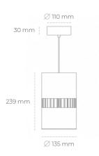
COB Light colour 4000 [K] | CRI 4350 [lm] Led chip flux Luminous flux 3480 [lm] System power 35 [W] Luminaire Efficiency 99 [lm/W] Beam angle ON/OFF Controller 3 SDCM MacAdam
