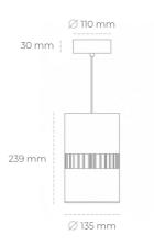
COB Light colour 3000 [K] | CRI Led chip flux 3227 [lm] Luminous flux 2581 [lm] System power 27 [W] Luminaire Efficiency 96 [lm/W] Beam angle 36° Controller ON/OFF MacAdam 3 SDCM
