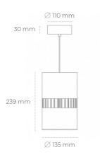
COB Light colour 2700 [K] | CRI Led chip flux 1111 [lm] Luminous flux 888 [lm] System power 10 [W] Luminaire Efficiency 89 [lm/W] Beam angle ON/OFF Controller 3 SDCM MacAdam
