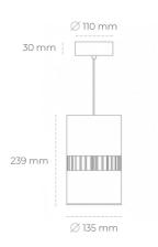
COB Light colour 5000 [K] | CRI 2895 [lm] Led chip flux Luminous flux 2316 [lm] System power 19 [W] 122 [lm/W] Luminaire Efficiency Beam angle 36° Controller ON/OFF MacAdam 3 SDCM
