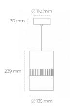
COB Light colour 3000 [K] | CRI Led chip flux 5172 [lm] Luminous flux 4137 [lm] System power 37 [W] Luminaire Efficiency 112 [lm/W] Beam angle 36° Controller ON/OFF MacAdam 3 SDCM
