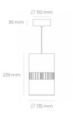
COB 4000 [K] HI EFFICIENT Light colour CRI 90 Led chip flux 3492 [lm] Luminous flux 2793 [lm] System power 21 [W] Luminaire Efficiency 133 [lm/W] Beam angle 36° Controller ON/OFF
