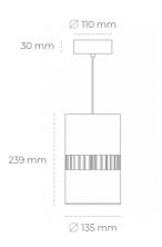
COB Light colour 5000 [K] | CRI Led chip flux 5502 [lm] Luminous flux 4401 [lm] System power 37 [W] Luminaire Efficiency 119 [lm/W] Beam angle 36° Controller ON/OFF MacAdam 3 SDCM
