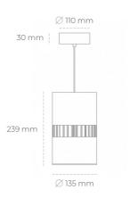
COB Light colour 2700 [K] | CRI Led chip flux 4311 [lm] Luminous flux 3448 [lm] System power 31 [W] Luminaire Efficiency 111 [lm/W] Beam angle 36° Controller ON/OFF MacAdam 3 SDCM
