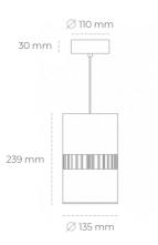
COB Light colour 2700 [K] | CRI 1886 [lm] Led chip flux Luminous flux 1508 [lm] System power 13 [W] Luminaire Efficiency 116 [lm/W] Beam angle 36° Controller ON/OFF MacAdam 3 SDCM
