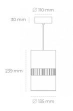
COB 3000 [K] HI EFFICIENT Light colour CRI 90 Led chip flux 1623 [lm] Luminous flux 1298 [lm] System power 10 [W] Luminaire Efficiency 130 [lm/W] Beam angle 36° Controller ON/OFF MacAdam
