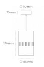
COB Light colour 4000 [K] | CRI 4591 [lm] Led chip flux Luminous flux 3672 [lm] System power 37 [W] Luminaire Efficiency 99 [lm/W] Beam angle 36° Controller ON/OFF MacAdam 3 SDCM
