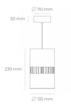
COB Light colour 3000 [K] | CRI 4380 [lm] Led chip flux Luminous flux 3504 [lm] System power 37 [W] Luminaire Efficiency 95 [lm/W] Beam angle 36° Controller ON/OFF MacAdam 3 SDCM
