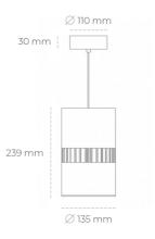
COB Light colour 3500 [K] | CRI Led chip flux 2783 [lm] Luminous flux 2226 [lm] System power 19 [W] Luminaire Efficiency 117 [lm/W] Beam angle 36° Controller ON/OFF MacAdam 3 SDCM
