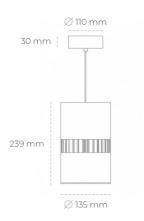
COB 3500 [K] HI EFFICIENT Light colour CRI 90 Led chip flux 3904 [lm] Luminous flux 3123 [lm] System power 25 [W] Luminaire Efficiency 125 [lm/W] Beam angle 36° Controller ON/OFF MacAdam
