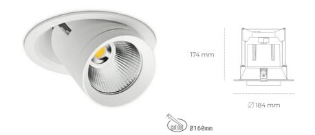
LED downlight for drop ceiling istallation. Aluminium housing. Glass cover included. Available in white, black and grey. Any RAL palette colour available on enquiry. Reflector beams available: 15°, 24°, 36°, 60°. Maximum power is 37W.
