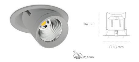
LED downlight for drop ceiling istallation. Aluminium housing. Glass cover included. Available in white, black and grey. Any RAL palette colour available on enquiry. Reflector beams available: 15°, 24°, 36°, 60°. Maximum power is 37W.
