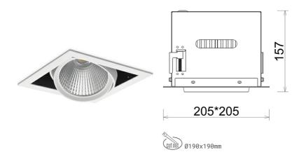
COB 2000 [K] MEAT PINK Light colour CRI Led chip flux 1253 [lm] Luminous flux 1002 [lm] System power 14 [W] Luminaire Efficiency 72 [lm/W] Beam angle 15° Controller ON/OFF MacAdam 3 SDCM
