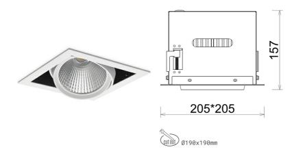
COB 2000 [K] MEAT PINK Light colour CRI Led chip flux 895 [lm] Luminous flux 716 [lm] System power 10 [W] Luminaire Efficiency 72 [Im/W] Beam angle 15° Controller ON/OFF MacAdam 3 SDCM
