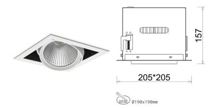
COB 3000 [K] CRI97 Light colour CRI Led chip flux 1575 [lm] Luminous flux 1260 [lm] System power 14 [W] Luminaire Efficiency 90 [lm/W] Beam angle 15° Controller ON/OFF MacAdam 3 SDCM
