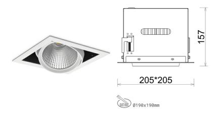
COB 5700 [K] SPECIAL Light colour CRI Led chip flux 4374 [lm] Luminous flux 3499 [lm] System power 35 [W] Luminaire Efficiency 100 [lm/W] Beam angle 45° Controller ON/OFF MacAdam 3 SDCM
