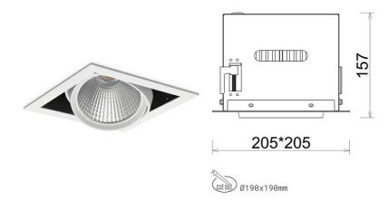
COB 5700 [K] SPECIAL Light colour CRI Led chip flux 4374 [lm] Luminous flux 3499 [lm] System power 35 [W] Luminaire Efficiency 100 [lm/W] Beam angle 30° Controller ON/OFF MacAdam
