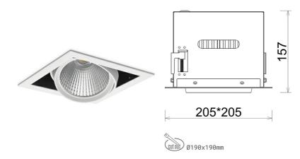
COB 4200 [K] MEAT WHITE Light colour CRI 90 Led chip flux 1976 [lm] Luminous flux 1580 [lm] System power 19 [W] Luminaire Efficiency 83 [lm/W] Beam angle 45° Controller ON/OFF MacAdam 3 SDCM
