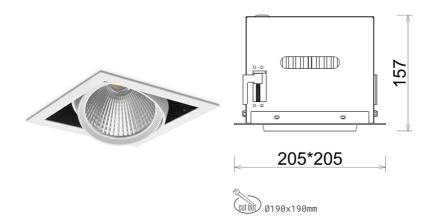
COB 4200 [K] MEAT WHITE Light colour CRI 90 Led chip flux 3539 [lm] Luminous flux 2831 [lm] System power 37 [W] Luminaire Efficiency 77 [Im/W] Beam angle 30° Controller ON/OFF MacAdam 3 SDCM
