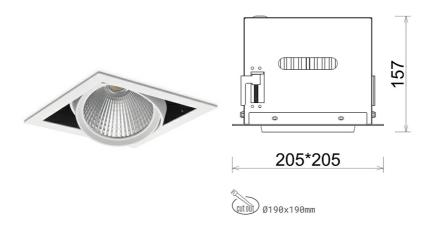
COB 4200 [K] MEAT WHITE Light colour CRI 90 Led chip flux 2695 [lm] Luminous flux 2156 [lm] System power 27 [W] Luminaire Efficiency 80 [lm/W] Beam angle 30° Controller ON/OFF MacAdam 3 SDCM
