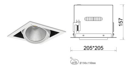
COB 4200 [K] MEAT WHITE Light colour CRI 90 Led chip flux 2519 [lm] Luminous flux 2015 [lm] System power 25 [W] Luminaire Efficiency 81 [lm/W] Beam angle 15° Controller ON/OFF MacAdam 3 SDCM
