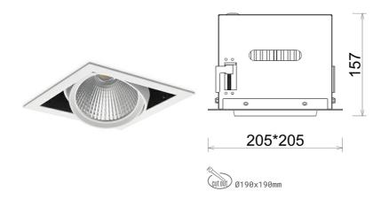
COB 4000 [K] HI EFFICIENT Light colour CRI 90 Led chip flux 5811 [lm] Luminous flux 4648 [lm] System power 36 [W] Luminaire Efficiency 129 [lm/W] Beam angle 30° Controller ON/OFF MacAdam 3 SDCM
