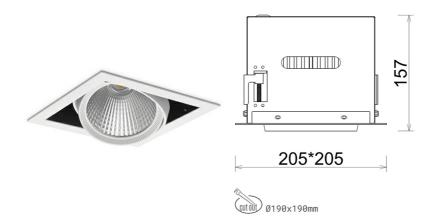
COB 4000 [K] HI EFFICIENT Light colour CRI 90 Led chip flux 4385 [lm] Luminous flux 3508 [lm] System power 27 [W] Luminaire Efficiency 130 [lm/W] Beam angle 30° Controller ON/OFF MacAdam 3 SDCM
