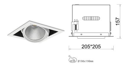
COB 3500 [K] HI EFFICIENT Light colour CRI 90 Led chip flux 4181 [lm] Luminous flux 3344 [lm] System power 27 [W] Luminaire Efficiency 124 [lm/W] Beam angle 45° Controller ON/OFF MacAdam 3 SDCM
