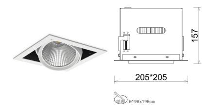
COB 3500 [K] HI EFFICIENT Light colour CRI 90 Led chip flux 3054 [lm] Luminous flux 2443 [lm] System power 19 [W] Luminaire Efficiency 129 [lm/W] Beam angle 30° Controller ON/OFF MacAdam 3 SDCM
