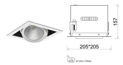
COB 3500 [K] HI EFFICIENT Light colour CRI 90 Led chip flux 4181 [lm] Luminous flux 3344 [lm] System power 27 [W] Luminaire Efficiency 124 [lm/W] Beam angle 15° Controller ON/OFF MacAdam 3 SDCM
