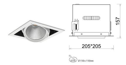
COB 3500 [K] HI EFFICIENT Light colour CRI 90 Led chip flux 1571 [lm] Luminous flux 1256 [lm] System power 10 [W] Luminaire Efficiency 126 [lm/W] Beam angle 15° Controller ON/OFF MacAdam 3 SDCM
