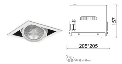
COB 3000 [K] HI EFFICIENT Light colour CRI 90 Led chip flux 4378 [lm] Luminous flux 3502 [lm] System power 27 [W] Luminaire Efficiency 130 [lm/W] Beam angle 60° Controller ON/OFF MacAdam 3 SDCM
