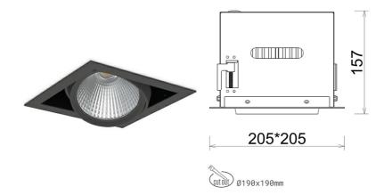
COB Light colour 4000 [K] | CRI Led chip flux 2658 [lm] Luminous flux 2126 [lm] System power 21 [W] Luminaire Efficiency 101 [lm/W] Beam angle 45° Controller ON/OFF MacAdam 3 SDCM
